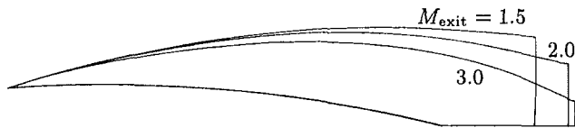
Fig. 8 Comparison of guide vane contours designed for different exit Mach numbers
